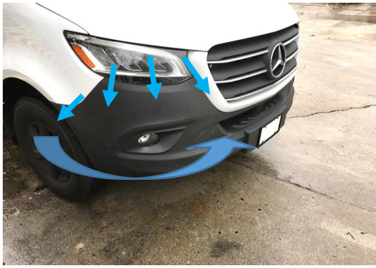
Figure 8: Removing Plastic Bumper
