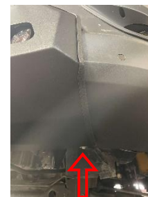
Figure 37: Lower Tray Mounting Bolt Location (Outside)
