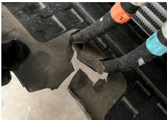
Figure 15: Air Flow Skirt Cut for Removal
