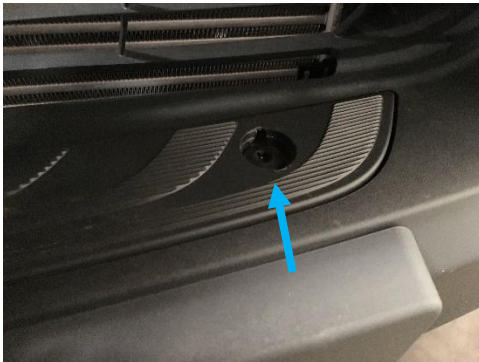
Figure 10: Front Bumper Step with Plastic Cap Removed
