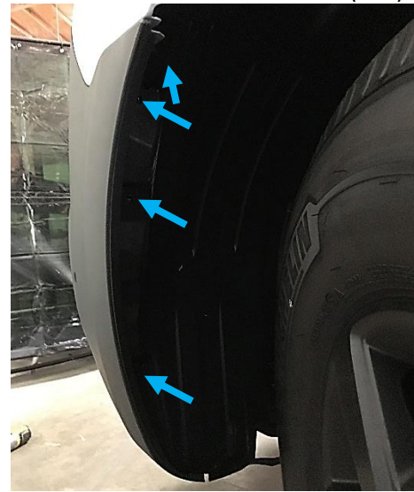
Figure 5: (4X) Plastic Rivets on the Inside of the Wheel Well
