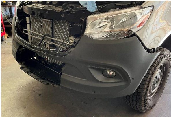
Figure 35: Loosely Installed Factory Front Bumper
