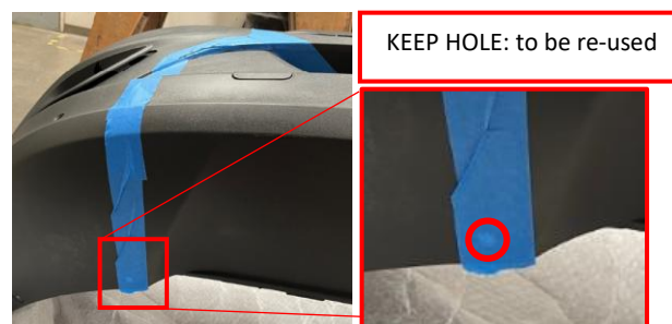
Figure 34: Bottom Mounting Location
