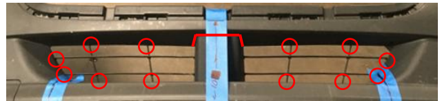
Figure 27: Cutout Grille Mesh from Air Flow Relief
