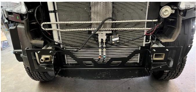
Figure 20: Winch tray Installed
