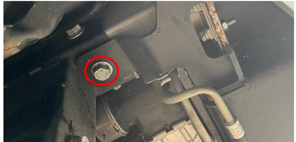
Figure 21: Installed Factory Crossmember Bolt Thru Winch Tray
