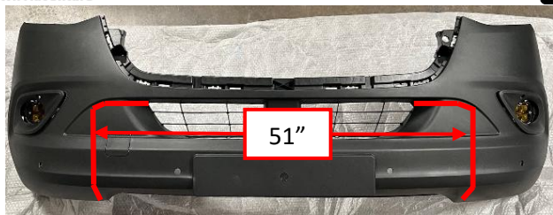
Figure 29: Marking Front Bumper Cutout
