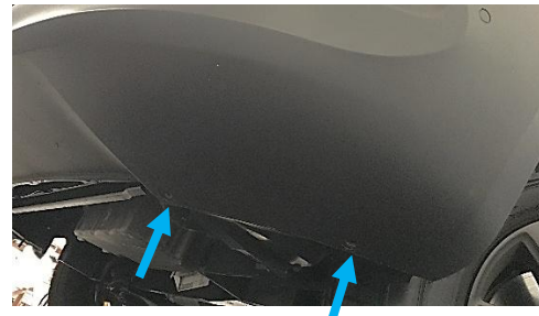
Figure 6: (2X) Plastic Rivets on Underside of Bumper
