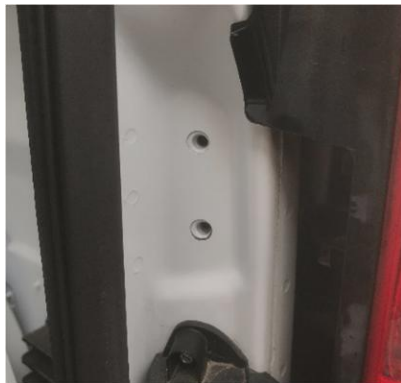
Figure 16: Factory Threaded Holes on Inside of Door Jam
