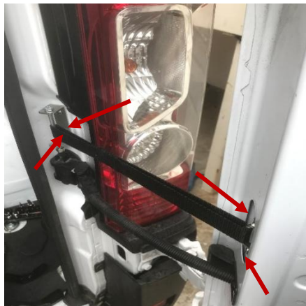
Figure 18: Completed Door Strap Installation
