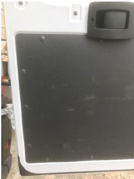
Figure 12: Remove Plastic Door Rivets
