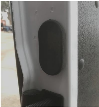
Figure 11: Remove Rubber Door Grommet
