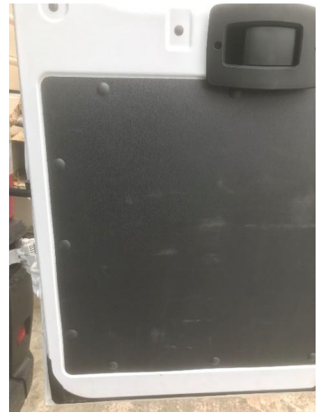
Figure 11: Remove Plastic Door Rivets
