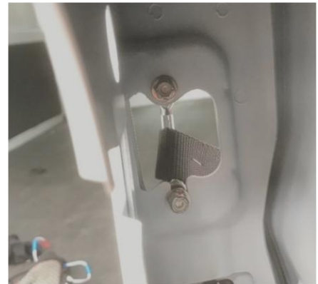
Figure 14: Backside View of Door Stop Mounting
