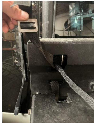
Figure 35: Webbing Anchor Pulled Through Pulley Holes
