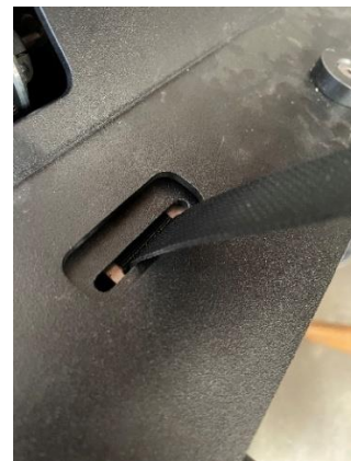
Figure 14: Webbing Anchor Installed Through Power Box Slit
