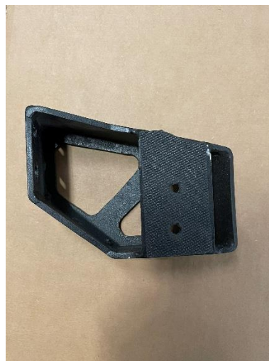
Figure 19: HD Lower Bracket with Foam Tape
