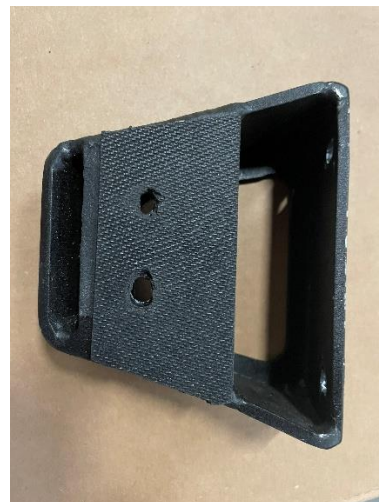
Figure 18: HD Upper Bracket with Foam Tape
