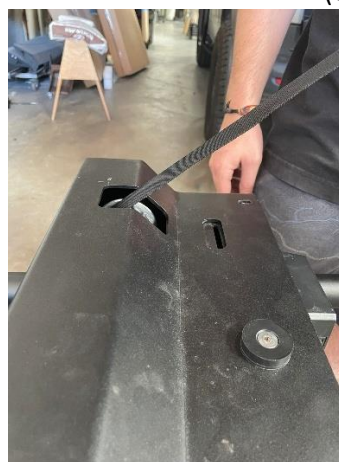
Figure 7: Threading Webbing Through Power Box Cover
