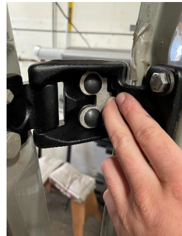
Figure 23: Upper Backing Plate Insertion
