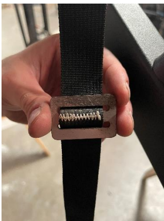
Figure 37: White Stitching Position on Webbing Anchors
