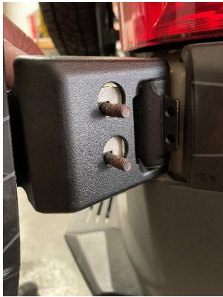
Figure 24: Lower Hinge Bolt Routing
