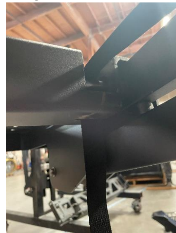
Figure 36: Webbing Threaded Over Pulley and Through Upper Tray Slot
