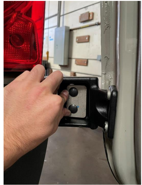
Figure 22: Lower Backing Plate Insertion
