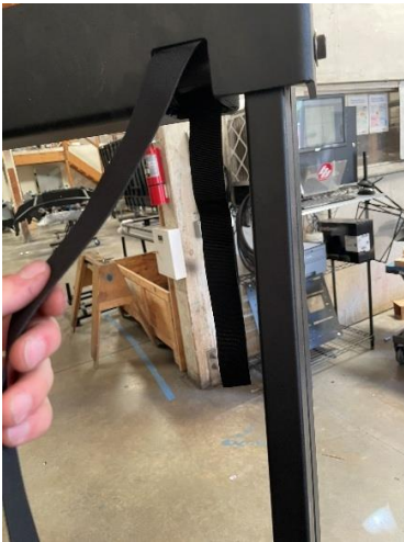
Figure 9: Threading Webbing Through Upper Tray Pulleys
