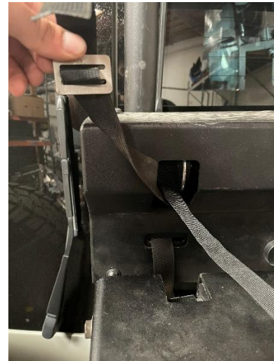
Figure 35: Webbing Anchor Pulled Through Pulley Holes
