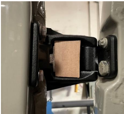
Figure 12: Cardboard to Push Bolts Out on Upper Hinge
