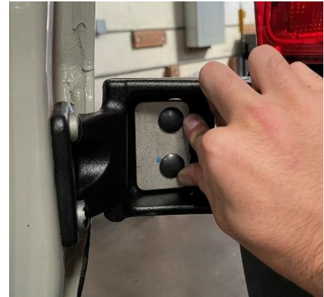
Figure 7: Lower Backing Plate Insertion
