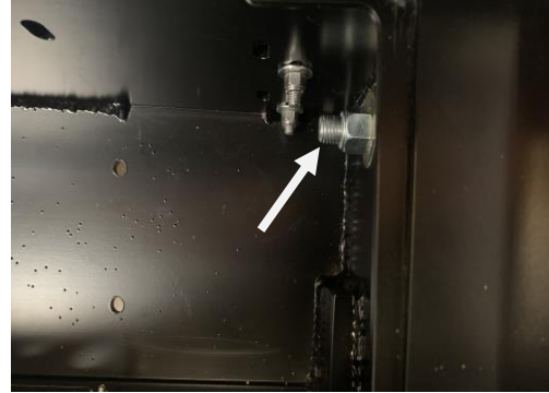
Figure 7: 1/2" hex bolt inside the toolbox
