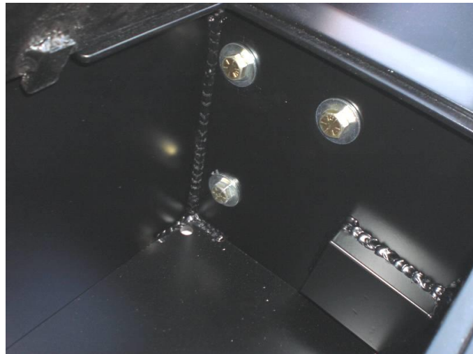
Figure 5: View of toolbox inside, showing correct orientation of mounting hardware
