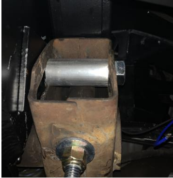
Figure 6: 1/2" hex bolt with crush tube
