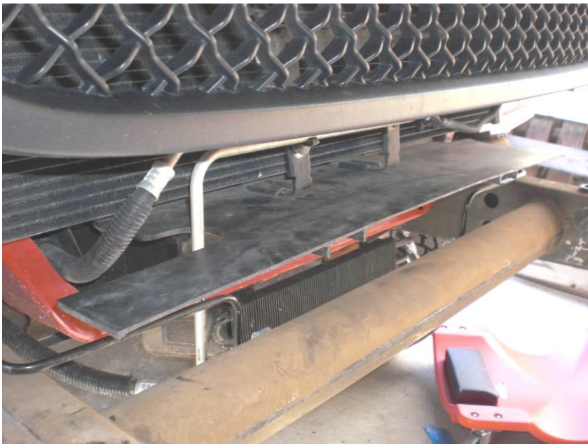
Figure 3: Trimmed plastic shield
