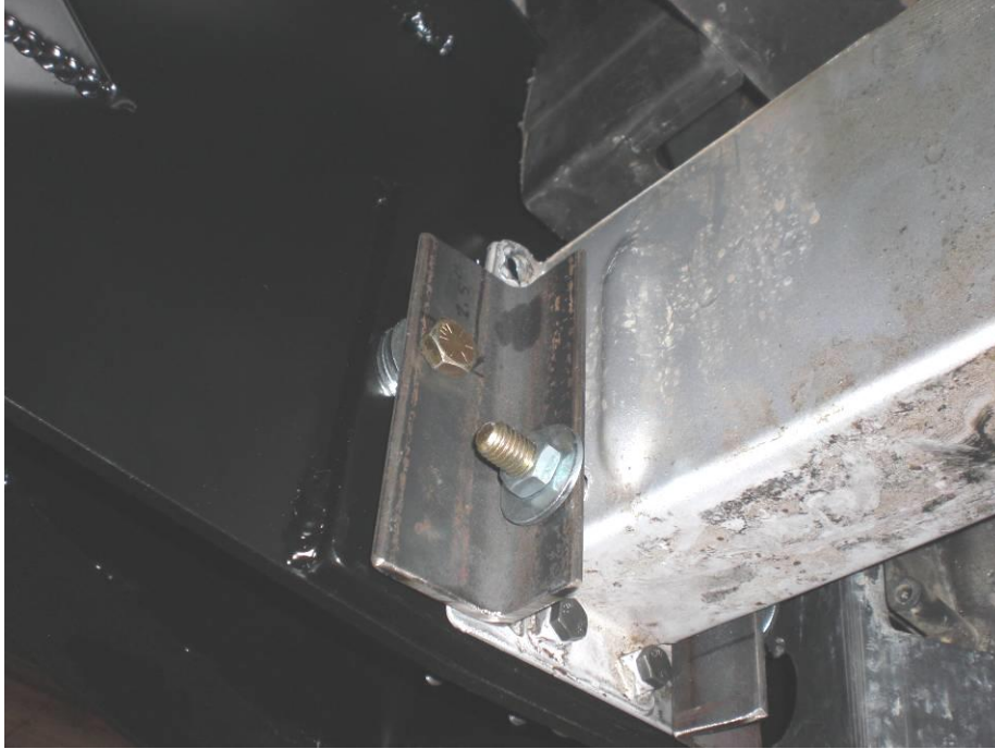
Figure 11: Steel support brackets bolted to frame
