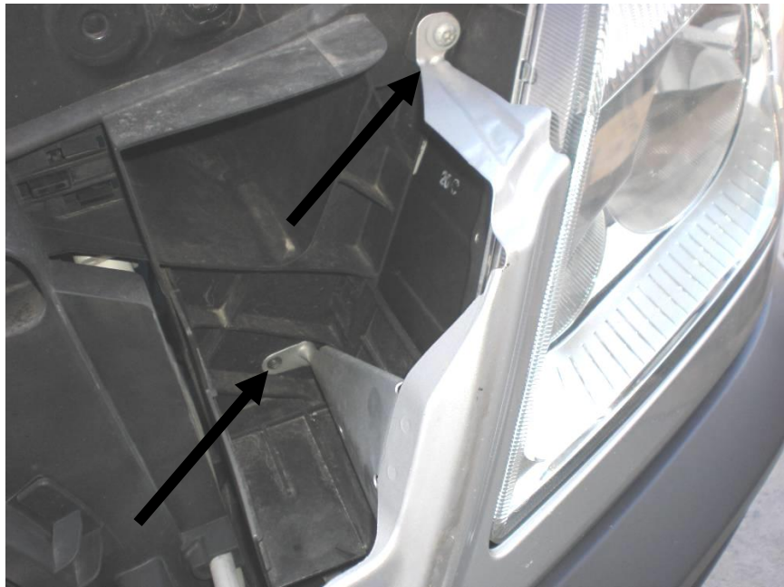
Figure 5: Headlight trim piece torx bolts
