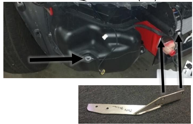
Figure 15: DEF Tank Bracket Placement
