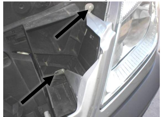
Figure 7: Headlight Trim Piece Torx Bolts
