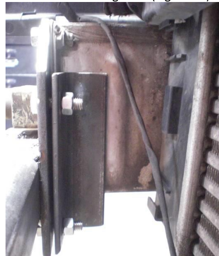
Figure 16: 2" X 1" Angle Brackets Attached to the Receiver Mounting Plate (This is the Passenger Side)
