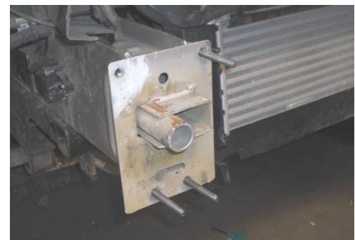
Figure 13: Frame Profile After Cutting
