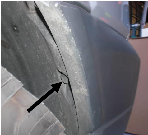
Figure 5: Plastic Fastener Location in Fender Well
