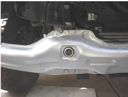
Figure 10: Stock Steel Bumper, Passenger Side
