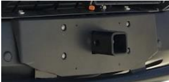
Figure 18: Verify Fitment of Front Receiver on Bumper and License Plate Cover
