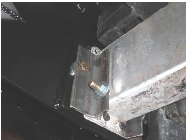
Figure 20: Steel support brackets bolted to frame
