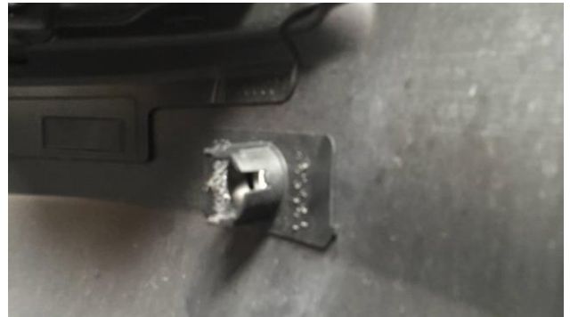
Figure 7. Sensor housing in the factory bumper.
