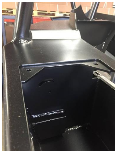
Figure 23. Install the crash sensor bracket in the orientation as shown.
