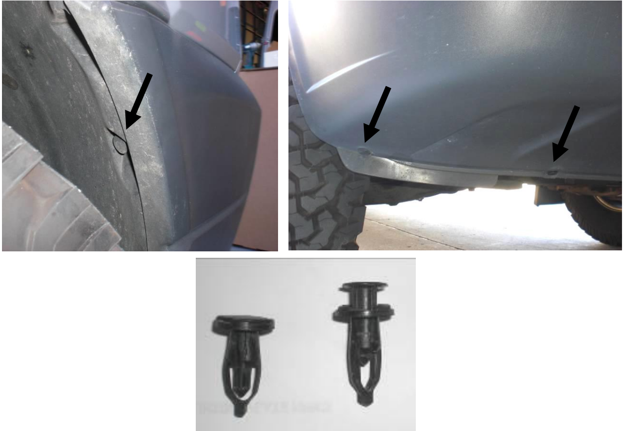
Figure 4: (Clockwise from top left) Plastic fastener location in fender well; Plastic fastener locations under leading edge of bumper; Plastic fastener closed (left) and open (right)
