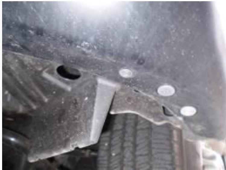
Figure 1. Remove 7 screws attaching the inner plastic fender.
