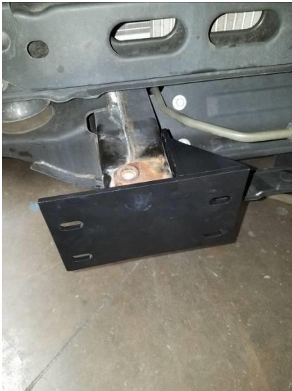
Figure 9a. Passenger side steel mounting bracket bolted onto frame. Note the orientation of the passenger vs driver side.
