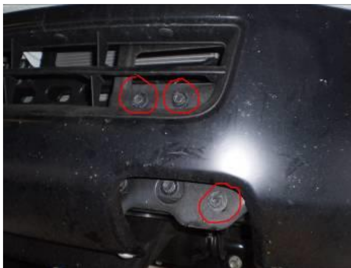
Figure 5. View from the front of the vehicle, 4 more bolts on the main bumper structure.
