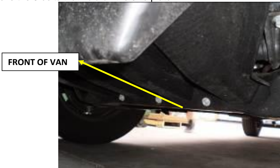
Figure 3. 6 bolts attaching the skid plate.
