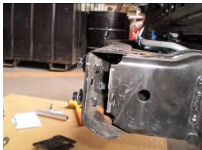
Figure 8a. Crossmember weld before cutting. Figure 8b. Crossmember weld after cutting.
