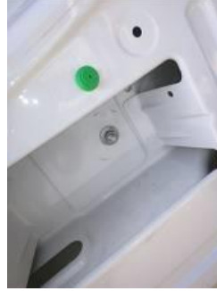
Figure 2. Door magnet bolt underneath door panels.
