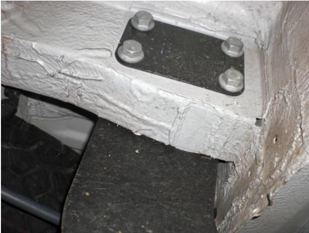
Figure 2: Aluminess Hitch with Factory Backing Plate on the Inside of the Frame
