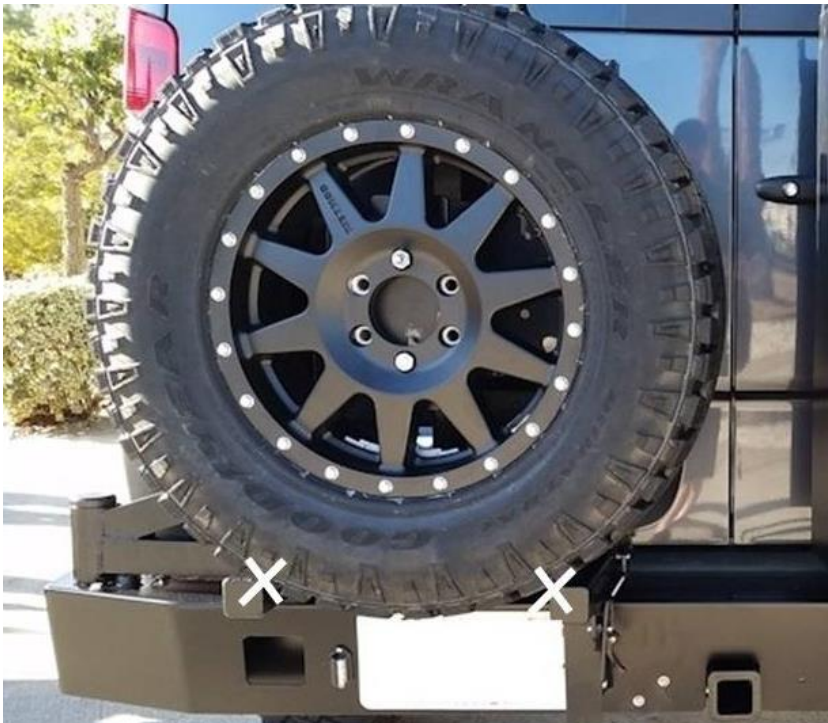
Figure 3. Rest tire on both support arms (before tightening the lugs or ubolts down).
