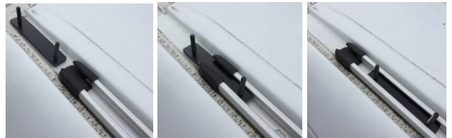
Figure 17: Studded Inserts Installed into Roof Tracks
