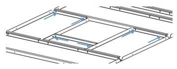
Figure 6: Bolting Vent Kit (NOTE: the small vent panel is only used for use with Fantastic Fans)
