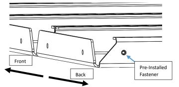
Figure 3: Close Up of Panel Orientation - Front-to-Back
