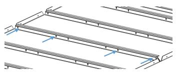
Figure 5: Bolting Panel-to-Panel (NOTE: the inner two holes are used only with the vent kit)
