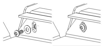
Figure 4: Example of Bolt Through Panels
