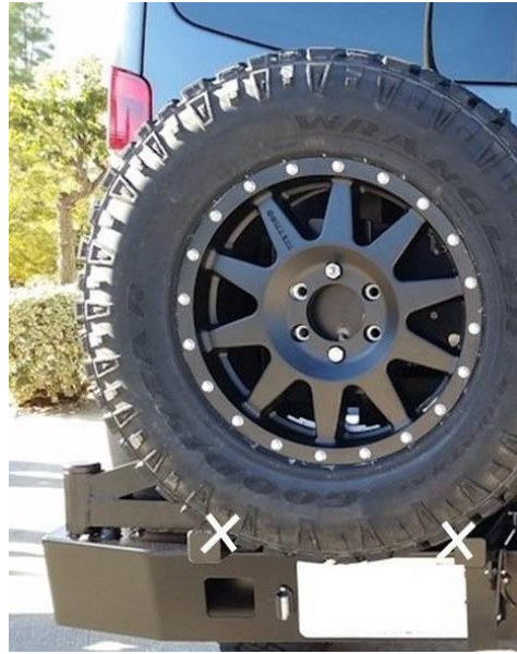
Figure 5. Rest tire on both support arms (before tightening the lugs or U-bolts down). If your tire is “floating” above these support arms, you may damage your swing arm while driving.
