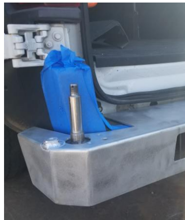
Figure 3. Tape applied to plastic corner pieces to prevent scratching. The swing arm has been removed and door is open to clearly show the location of the tape, although THIS IS NOT THE CONFIGURATION IN WHICH YOU SHOULD INSTALL YOUR ALUMINESS BUMPER.
