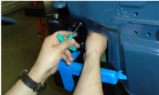
Figure 12: Tightening Hardware Through Insert Opening
