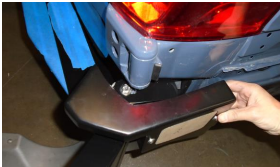
Figure 13: Installation of the Trim Assembly
