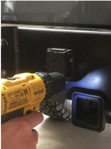
Figure 15: Installation of the trailer plug
