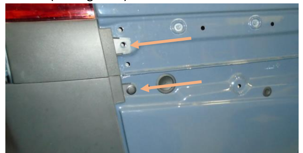
Figure 6: Plastic Rivets Underneath the Side Panel
