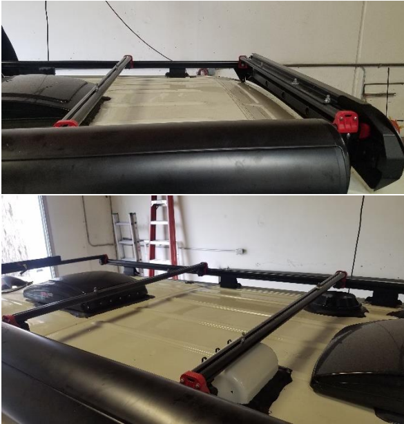
Figure 1. Solar Panels removed from stock rack.
