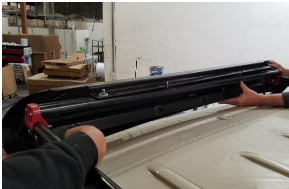
Figure 5. Remove front panel and set light bar aside.
