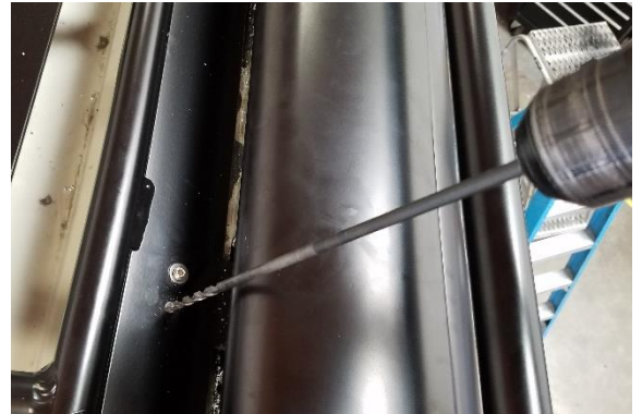
Figure 11. Drill holes above the mounting brackets and bolt together one at a time to install the roof rack on the awning side of your vehicle.
