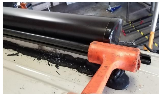
Figure 8. Remove passenger side rail.
