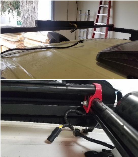
Figure 2. Electrical accessories disconnected.
