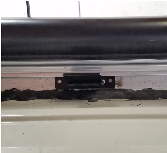
Figure 9. Awning channel bracket in awning track.
