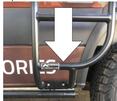
Figure 4: Lower Attachment Assembly
