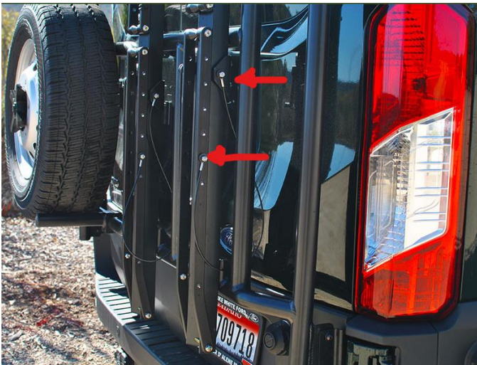
Figure 8: Steel Cable Location
