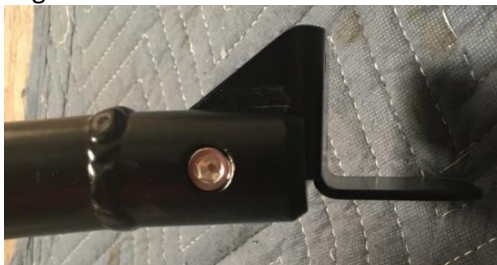
Figure 2: Ladder Attachment to Upper Brackets
