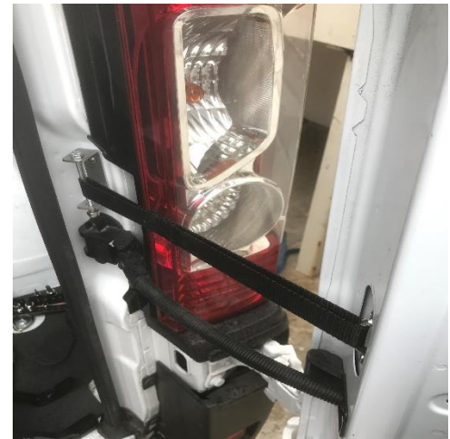
Figure 23: Complete Door Stop Install
