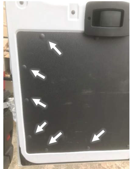
Figure 18: Remove Plastic Door Rivets
