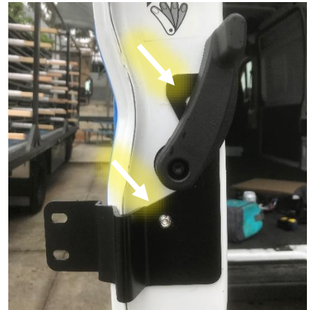
Figure 12: Inner Driver Door Bracket Installed
