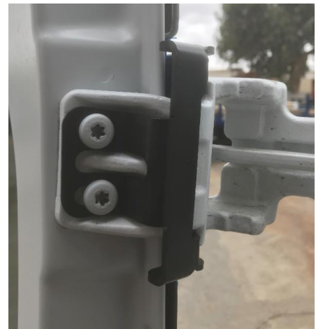
Figure 7: Inside View of Installed Upper Hinge Bracket
