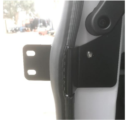
Figure 15: Installed Weather Stripping After Modification
