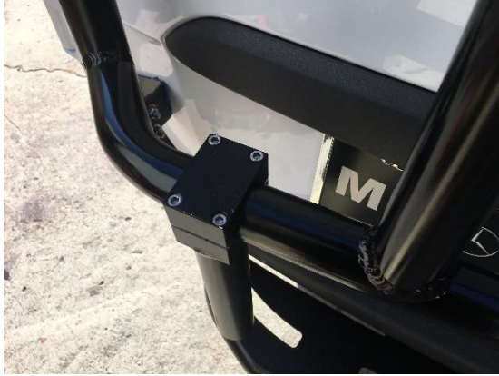
Figure 9: Bolt-On Supports Loosely Bolted to Lower Crossmember
