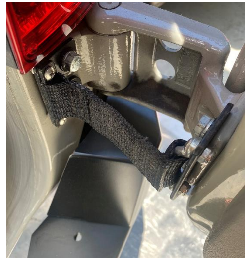
Figure 10: Limiting Strap Installed
