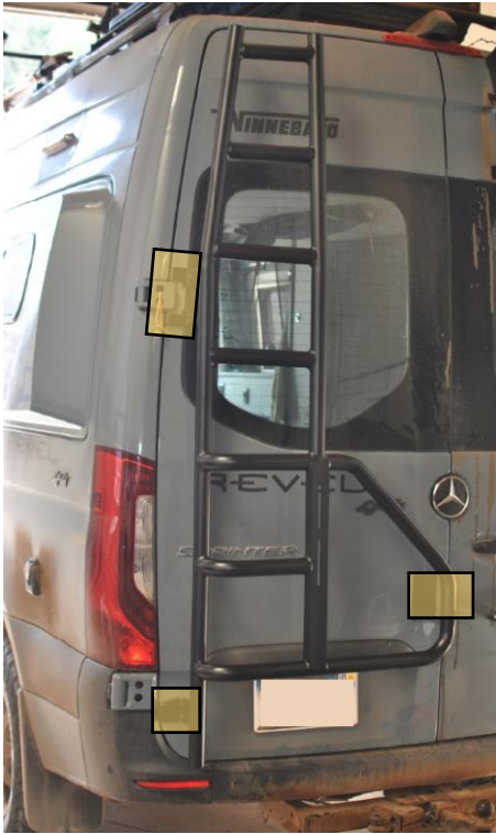
Figure 3: Protective Tape Locations on Door
