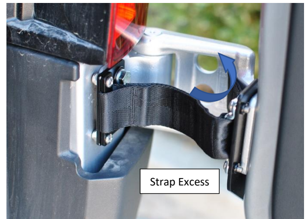
Figure 8: Adjustable Limiting Strap Installed
