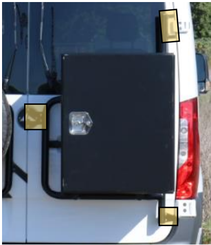
Figure 1: Protective Tape Locations on Door
