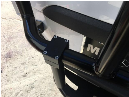
Figure 1: Bolt-On Supports Loosely Bolted to Lower Crossmember
