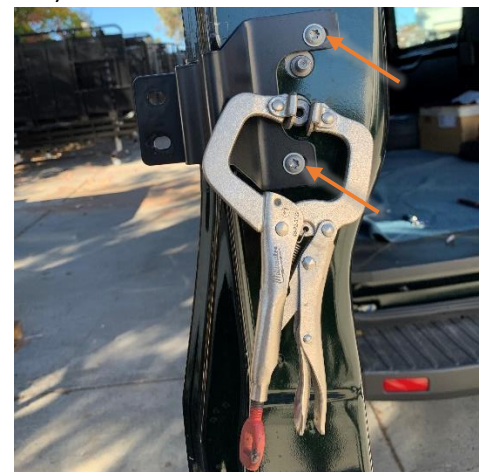
Figure 8: Inner Driver Door Bracket Installed
