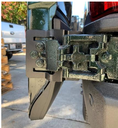
Figure 5: Inside View of Installed Lower Hinge Bracket
