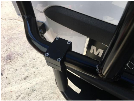
Figure 14: Bolt-On Supports Loosely Bolted to Lower Crossmember
