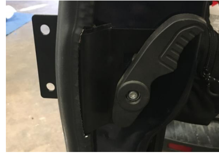
Figure 12: Installed Weather Stripping After Modification
