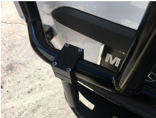
Figure 14: Bolt-On Supports Loosely Bolted to Lower Crossmember
