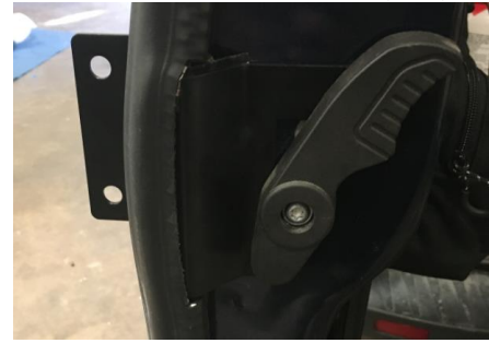
Figure 12: Installed Weather Stripping After Modification
