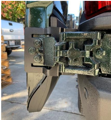
Figure 5: Inside View of Installed Lower Hinge Bracket
