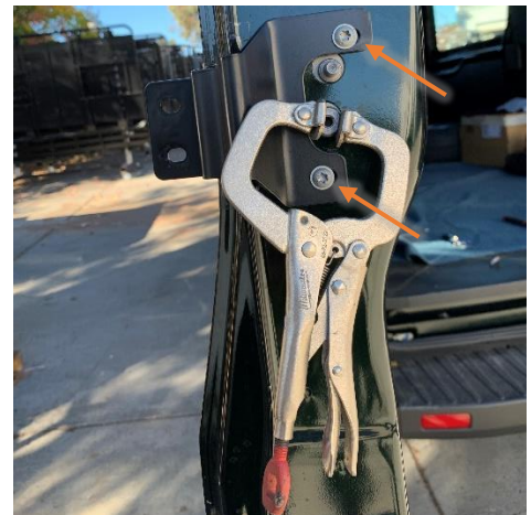
Figure 8: Inner Driver Door Bracket Installed
