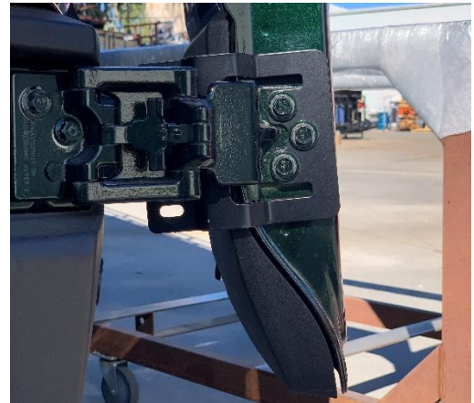
Figure 4: Inside View of Installed Lower Hinge Bracket
