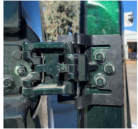
Figure 4: Inside View of Installed Upper Hinge Bracket
