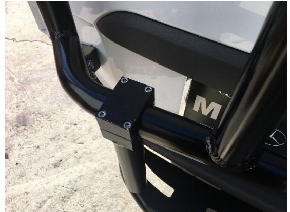
Figure 8: Bolt-On Supports Loosely Bolted to Lower Crossmember
