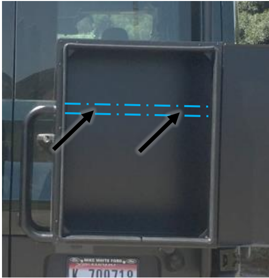
Figure 10: Mounting Box to Upper Cross Bar
