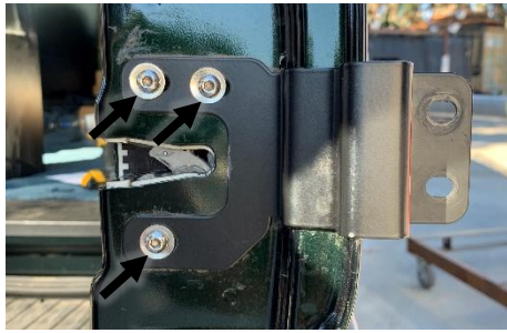
Figure 6: Installed Inner Passenger Door Bracket
