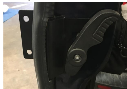
Figure 12: Installed Weather Stripping After Modification
