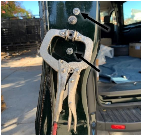
Figure 8: Inner Driver Door Bracket Installed
