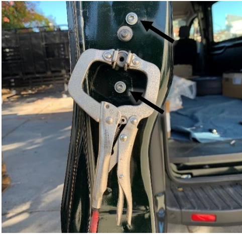
Figure 7: Inner Door Bracket Installed
