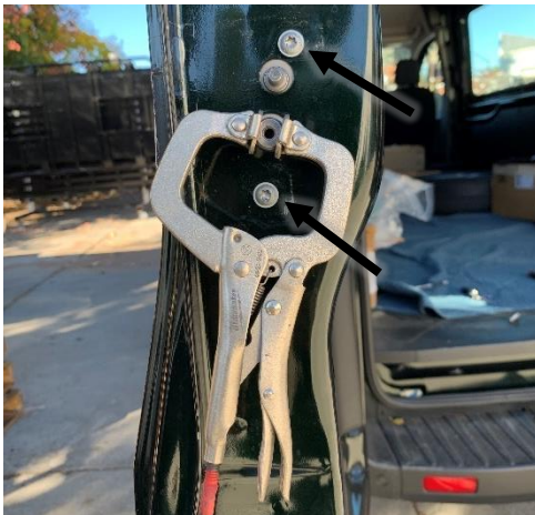
Figure 8: Inner Driver Door Bracket Installed
