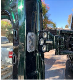
Figure 2: Upper Hinge Rotated Away from Door
