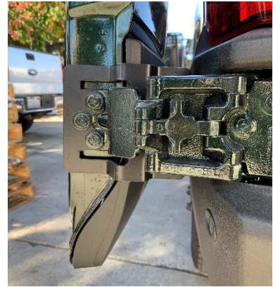
Figure 5: Inside View of Installed Lower Hinge Bracket
