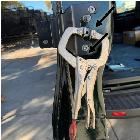
Figure 8 Inner Driver Door Bracket Installed
