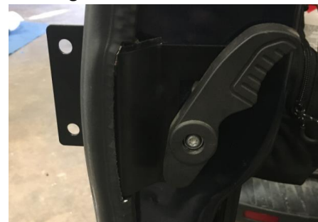
Figure 12: Installed Weather Stripping After Modification
