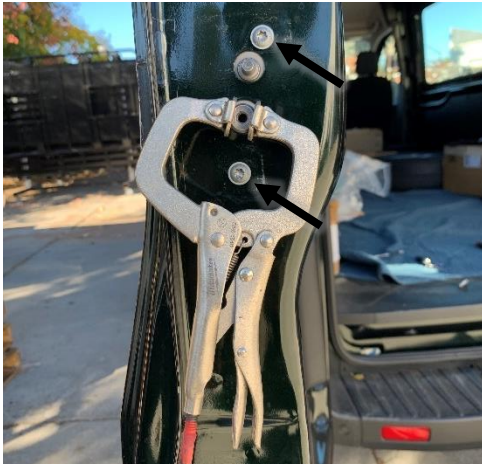
Figure 7: Removing Factory Torx Screws
