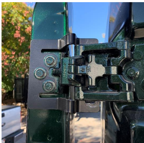
Figure 4: Inside View of Installed Upper Hinge Bracket
