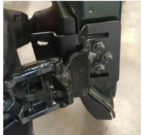
Figure 6: Inside View of Installed Lower Hinge Bracket
