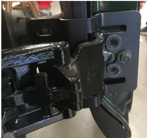
Figure 4: Hinge Placed Back into Position
