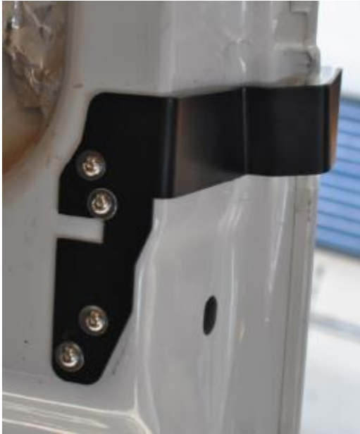
Figure 12: Installed Inside Upper Bracket without Factory Handle
