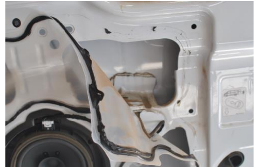
Figure 10: Inner Door Liner Peeled Back for Access
