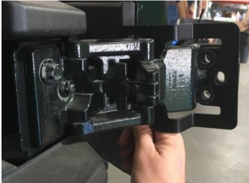
Figure 3: Bracket Installed Over Factory Hinge
