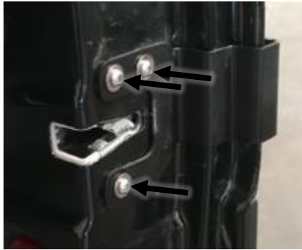
Figure 8: Installed Inner Passenger Door Bracket
