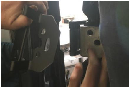
Figure 2: Upper Hinge Rotated Away from Door
