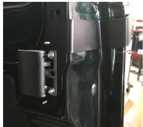
Figure 15: Upper Inner Passenger's Side Bracket Installed
