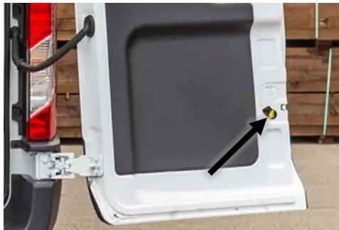
Figure 7: Inside Latch on Passenger Door
