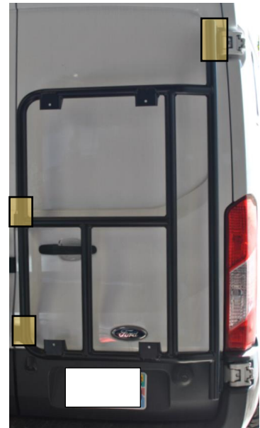
Figure 1: Locations of Protective Film Application
