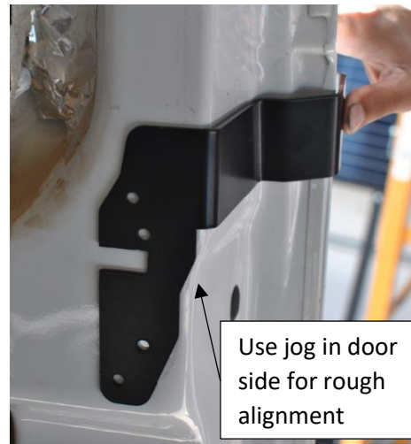
Figure 11: Dry Fit Bracket Up to Door
