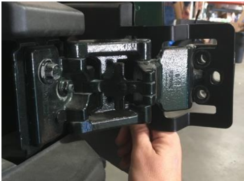
Figure 3: Bracket Installed Over Factory Hinge
