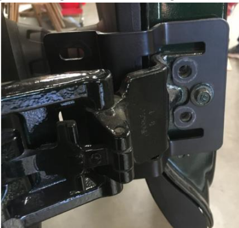
Figure 4: Hinge Placed Back into Position
