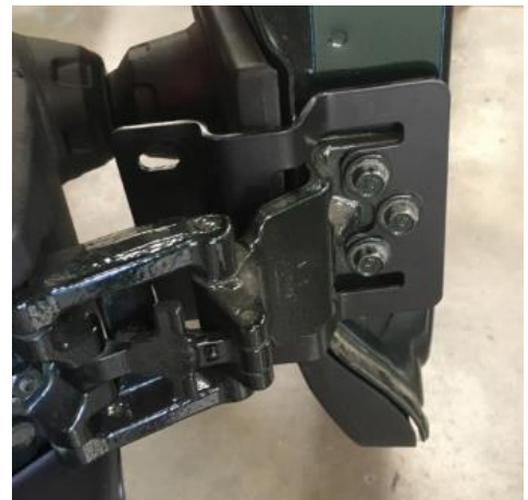
Figure 6: Inside View of Installed Lower Hinge Bracket
