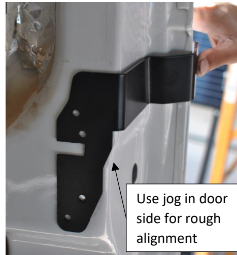
Figure 11: Dry Fit Bracket Up to Door
