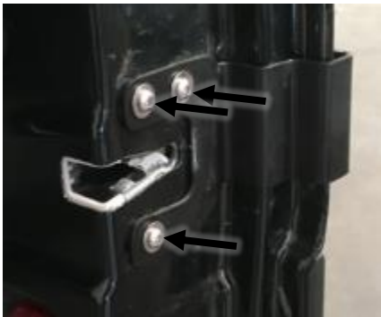
Figure 8: Installed Inner Passenger Door Bracket
