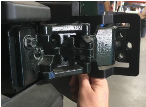
Figure 3: Bracket Installed Over Factory Hinge
