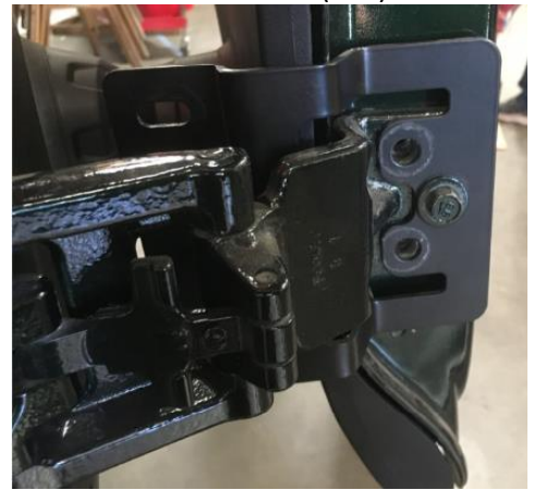
Figure 4: Hinge Placed Back into Position
