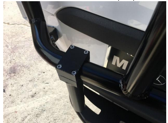
Figure 7: Bolt-On Supports Loosely Bolted to Lower Crossmember
