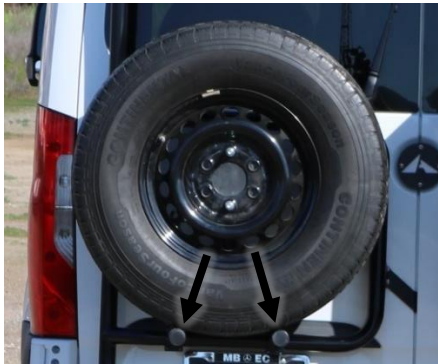
Figure 10: Tire Resting on Tire Supports
