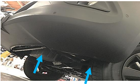
Figure 8: Plastic Rivets on Underside of Bumper
