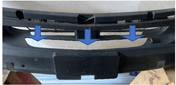
Figure 27: Factory Front Step Removal
