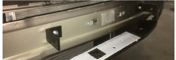
Figure 13: Attachment Brackets Attached to Sub-Frame
