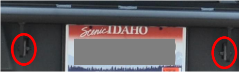
Figure 16: Upper subframe attachment locations
