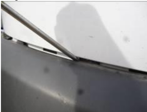
Figure 9: Prying Front Bumper from Grille
