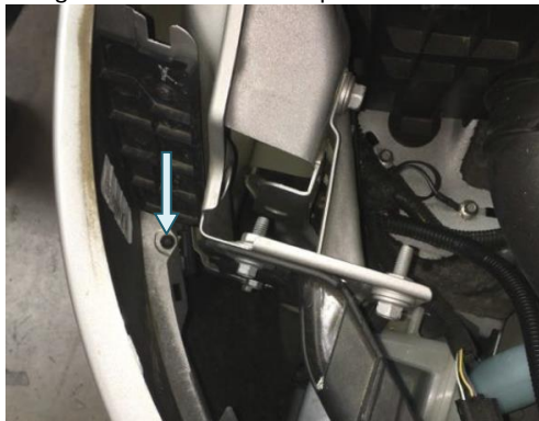
Figure 2: Bolts Underneath the Headlights
