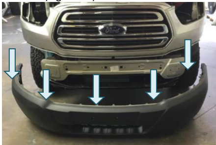
Figure 10: Front Bumper Removal
