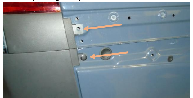
Figure 6: Plastic Rivets Underneath the Side Panel
