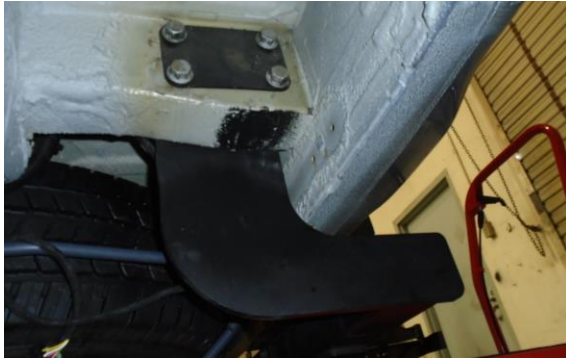
Figure 1: Four (4) of the Hitch Mounting Bolts
