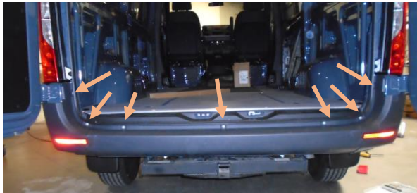
Figure 2: Torx Bolts on the Rear Bumper
