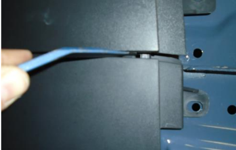
Figure 7: Removing Small Plastic Panel from Rear Bumper
