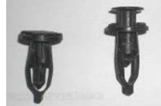
Figure 3: Plastic Rivets Underneath Bumper
