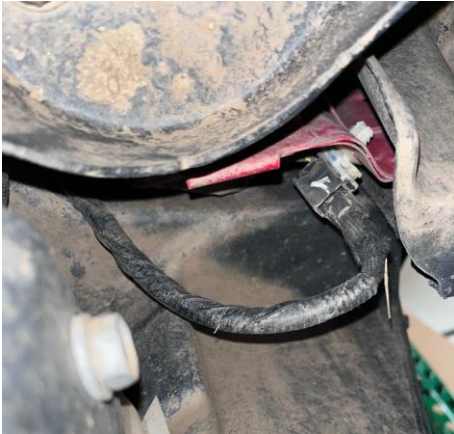
Figure 1: Skid Plate Bolt Location
