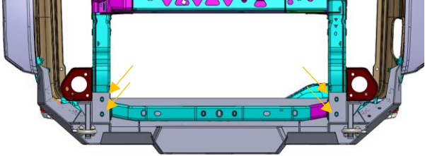
Figure 7: Bolt Bumper to Frame through Slots
