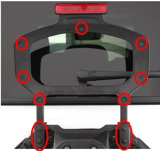
Figure 6: Accessing 3 rd Brake Light Wiring Harness
