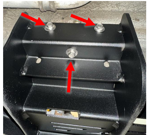
Figure 6: Step Bracket Installation Behind Pinch Weld
