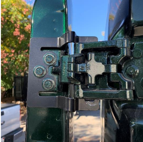
Figure 4: Inside View of Installed Upper Hinge Bracket
