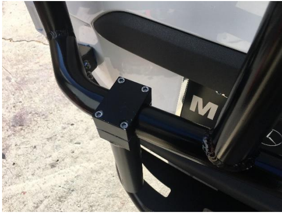
Figure 4: Bolt-On Supports Loosely Bolted to Lower Crossmember
