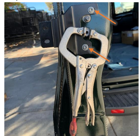
Figure 8: Inner Driver Door Bracket Installed
