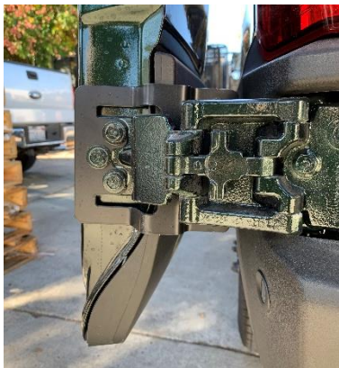
Figure 5: Inside View of Installed Lower Hinge Bracket
