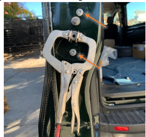
Figure 7: Removing Factory Torx Screws
