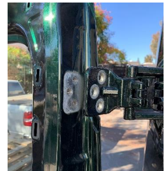
Figure 2: Upper Hinge Rotated Away from Door
