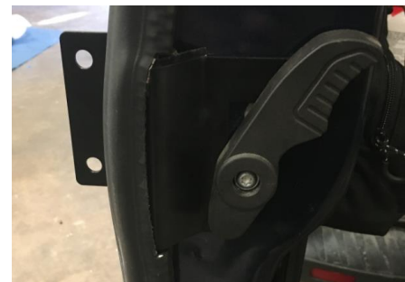
Figure 12: Installed Weather Stripping After Modification
