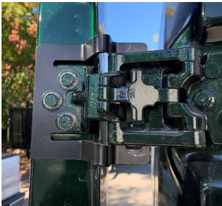
Figure 4: Inside View of Installed Upper Hinge Bracket
