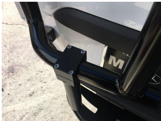
Figure 4: Bolt-On Supports Loosely Bolted to Lower Crossmember
