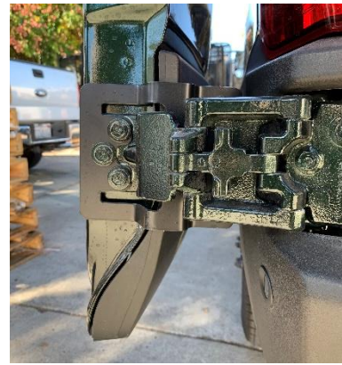
Figure 5: Inside View of Installed Lower Hinge Bracket
