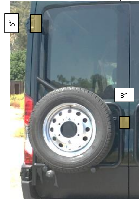
Figure 1: Locations of Protective Film Application
