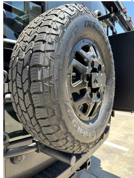
Figure 5: Tire Mount Assembled
