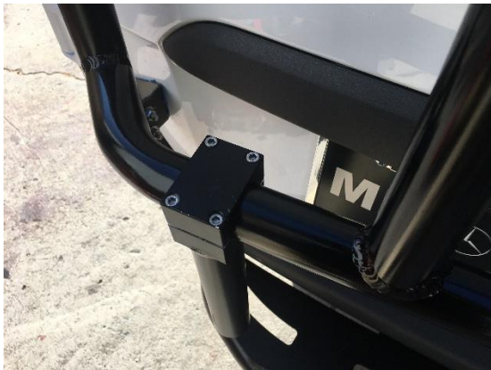
Figure 1: Bolt-On Supports Loosely Bolted to Lower Crossmember
