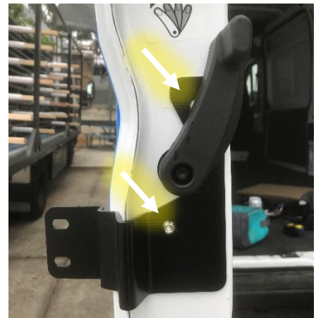
Figure 12: Inner Driver Door Bracket Installed
