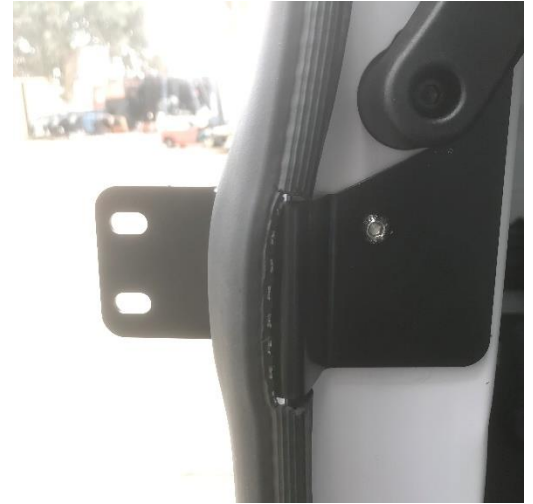
Figure 15: Installed Weather Stripping After Modification
