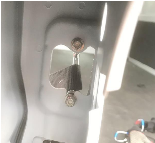
Figure 21: Backside View of Door Stop Mounting
