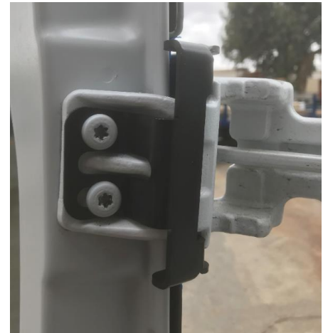
Figure 7: Inside View of Installed Upper Hinge Bracket
