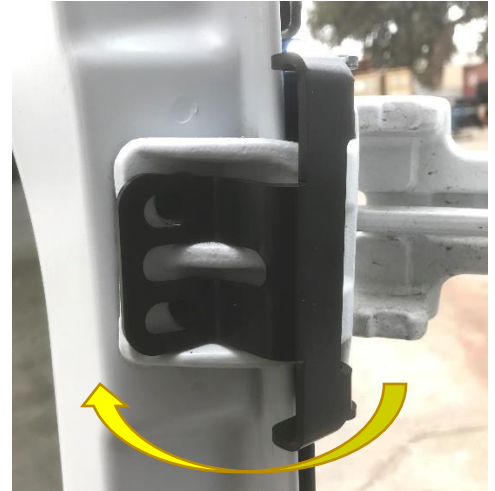
Figure 6: Bracket Installed Over Factory Hinge
