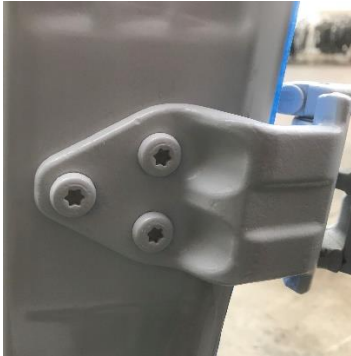
Figure 8: Inside View of Lower Hinge
