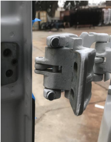
Figure 4: Upper Hinge Rotated Away from Door
