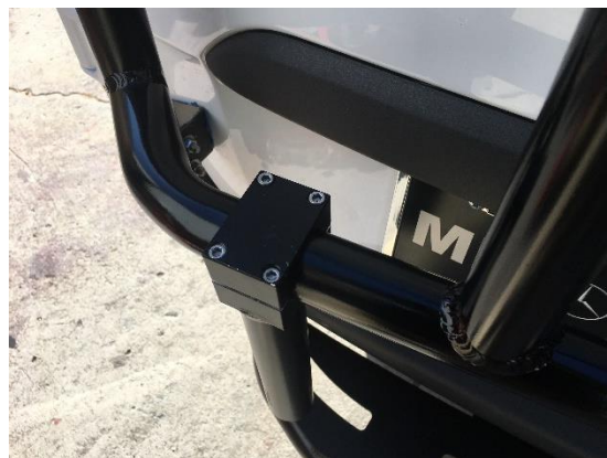
Figure 1: Bolt-On Supports Loosely Bolted to Lower Crossmember
