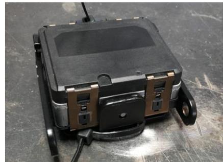
Figure 11: Tighten Zip Tie(s) Around Top of Sensor Carriage
