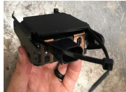
Figure 9: Feed a Zip Tie Between the Sensor and Sensor Carriage (Behind Sensor)
